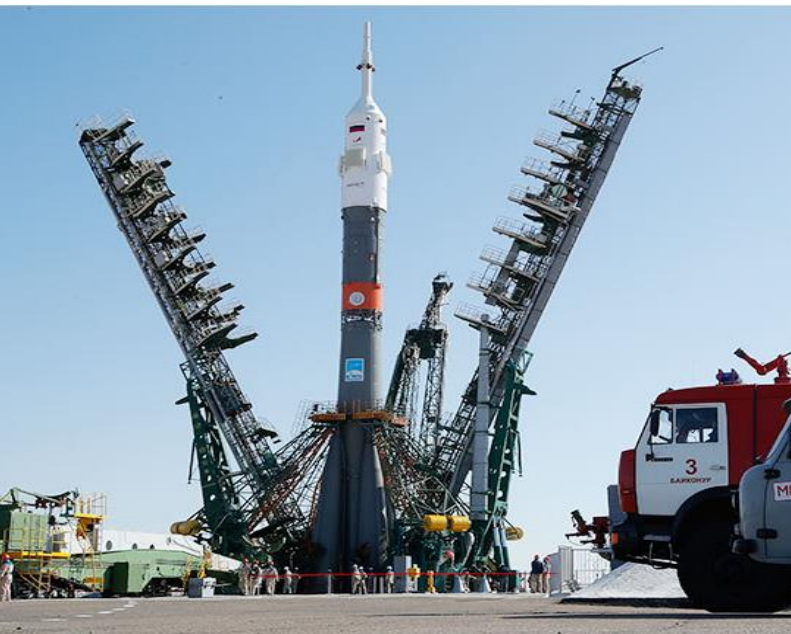
The Soyuz booster rocket FG with Soyuz MS-15 spacecraft is mounted on the launch pad.
